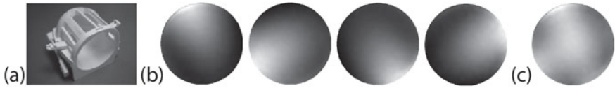
Figure 1.11: RF-receiver coil array with sensitivity maps. (a) Twelve-channel head receiver coil array for a MAGNETOM Trio, A Tim System 3T, Siemens Healthcare, Erlangen, Germany. (b) Four RF-coil sensitivity maps at 3 T of the coil shown in (a), where each map has been combined from three others. The maps were determined by dividing images of each receiver channel, acquired with a homogeneous phantom, by the corresponding RF-transmit field maps, which were measured similar to the method described in [34]. (c) Root-sum-of-squares image of the RF-sensitivity profiles.
