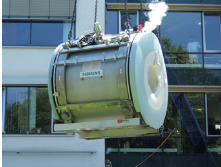
Figure 1.1: This MR scanner (MAGNETOM Trio, A Tim System 3T, Siemens Healthcare, Erlangen, Germany) was equipped with a PatLoc insert coil while this thesis was conducted. The scanner is shown during delivery to the site of installation. Visible from outside is the vacuum chamber that contains the main magnet, the largest component of the scanner.
