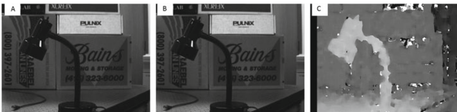
Fig. 6. Generation disparity map. The left (A) and middle (B) are stereo images. Right (C) is the disparity map
