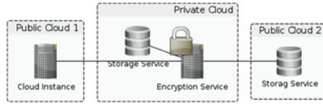
Fig. 1. Encryption service usable by end users to secure data before they are stored in a public cloud.
