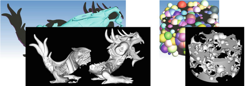
Fig. 5. LTR: Asian Dragon minus Happy Buddha (8,306,513 triangles) and cylinder minus 1,000 random spheres (5,177,870 triangles), both original volumes and ray casted Boolean subtraction result.
