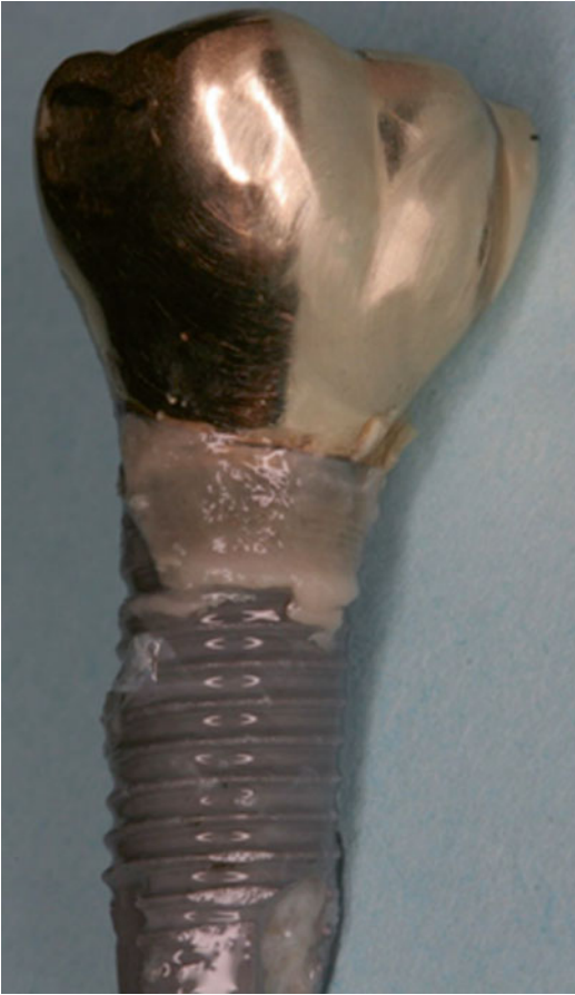
Fig. 2.7 Example of a failed implant with residual excess cement. XRF analysis determined this as RelyX luting cement
