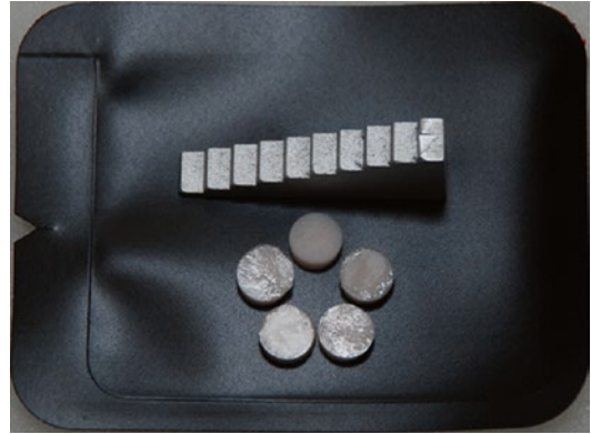
Fig. 5.4 Specimen disks with modified step wedge
