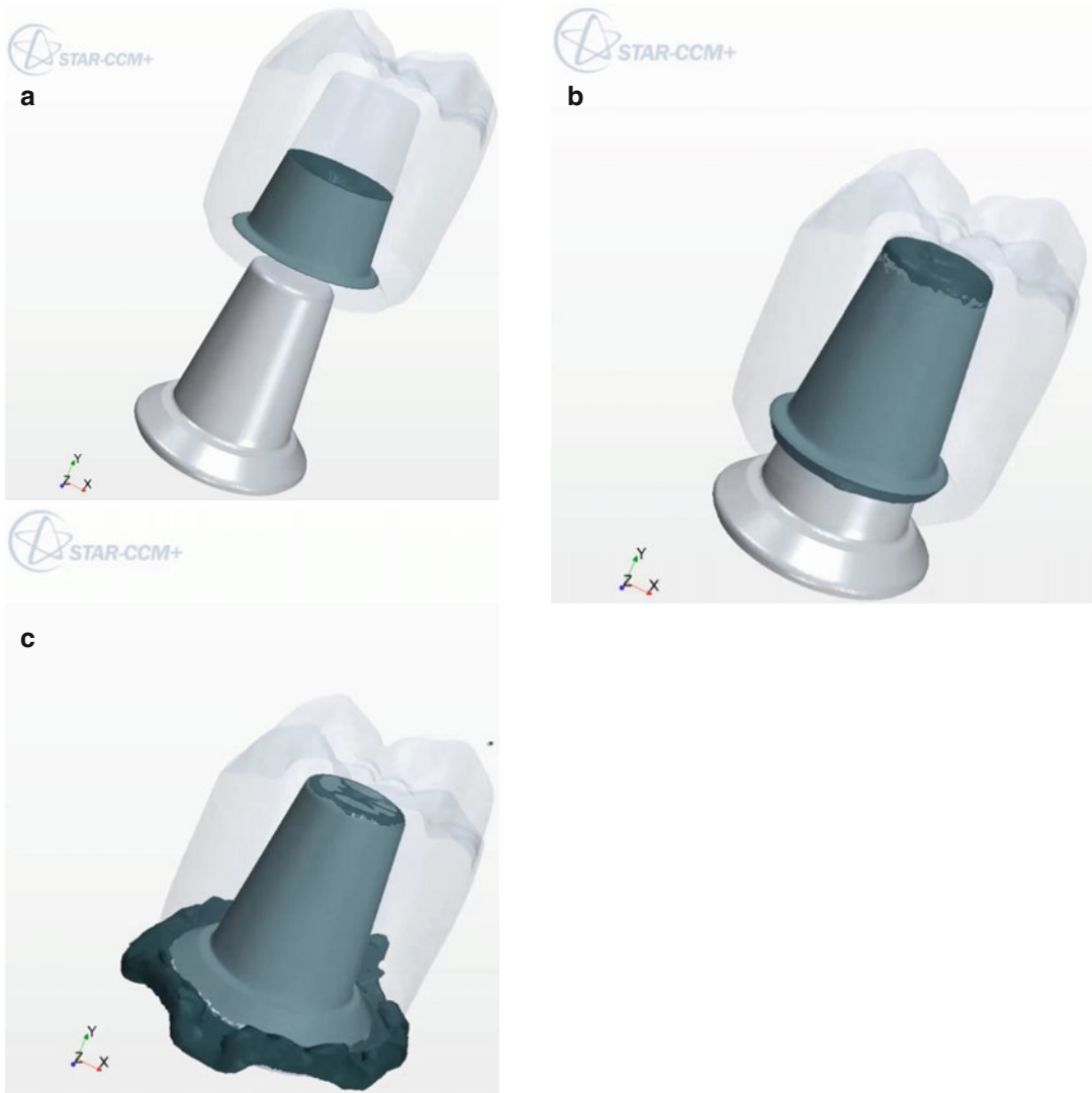
Fig. 4.37 (a–c) Clip images from 3-D animation of the crown seating on the abutment and resultant cement flow: (a) start; (b) 3/4 seat; (c) full seat with cement extrusion
