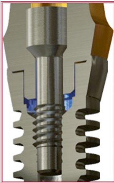
Fig. 7.28 Conus connection: the contacting planes between implant and abutment. There is no actual contact between hex and implant
