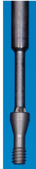
Fig. 9.11 A screwdriver (Straumann) engages the head of an implant screw. Note how the shank of the screwdriver lies in the same long axial planes, acting as an extension of the screw
