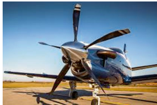
Fig. 4.21 A propeller nose cone forces air to either side and onto the blades of the prop
