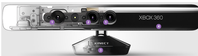
Fig. 3. Composition of the Kinect sensor: (1) - Infrared optics; (2) - RGB camera; (3) - Motorized tilt; (4) - Multi-array microphone [4]
