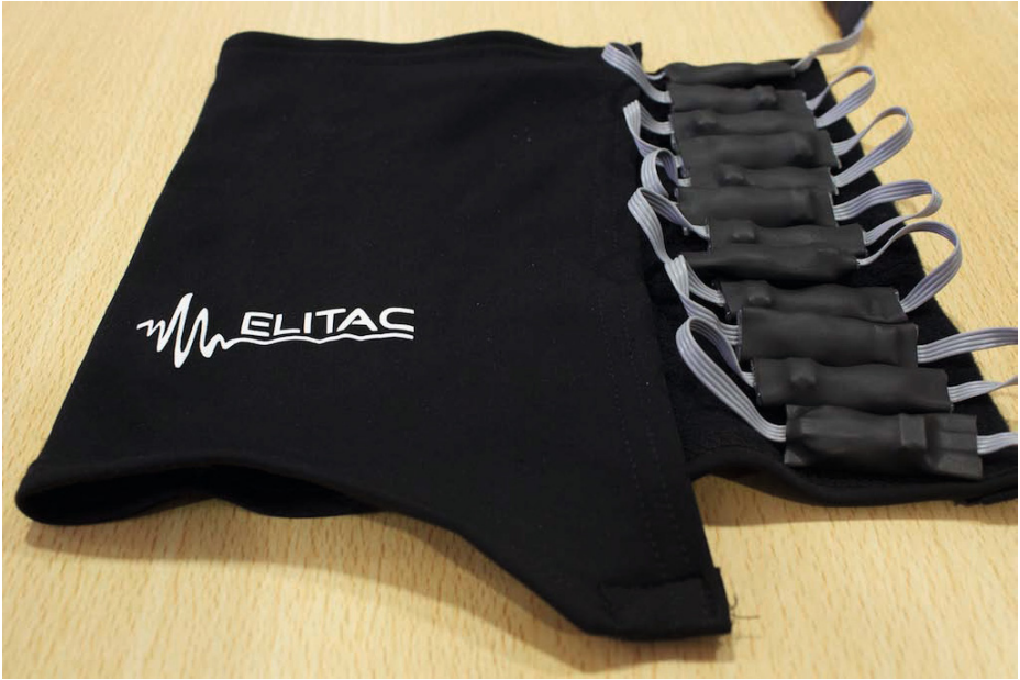
Fig. 3. The vibrotactile sleeve with 12 vibrationmotors
