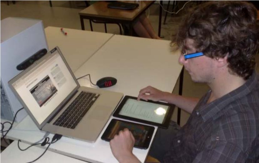
Fig. 9. Experimental setup: videos are displayed on a computer screen while the user needs to play a game and answer questions simultaneously. A 3D sensor on top of the screen captures the head movement of the user.
