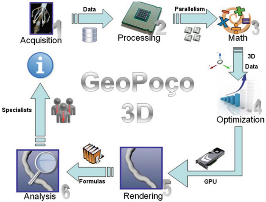
Fig. 13.3 The framework of the 3D Caliper tool (GeoPoço 3D)
