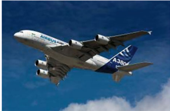
Fig. 13.5 Airbus A380 with maximum take-off weight of approx. 560 t, in use since 2007 (Photograph [7])
