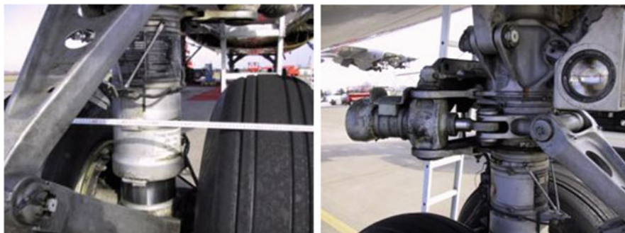
Fig. 14.16 Massive structure of the nose tire including steering mechanism
