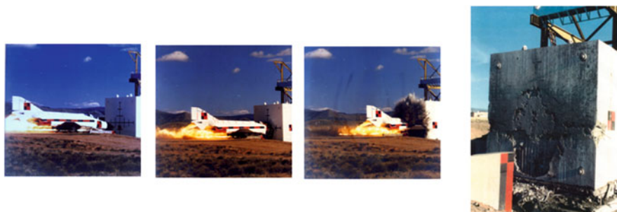
Fig. 14.9 Pictures of the large scale experiment with a Phantom at the Sandia National Laboratories in the USA in 1988; the target body after the impact on the right
