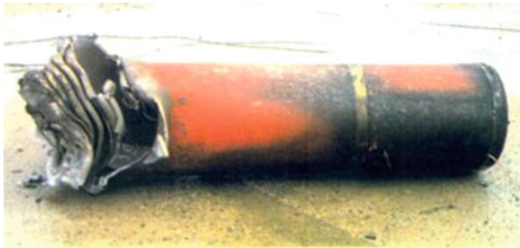
Fig. 14.7 Projectile after impact (soft impact, experiments in Meppen)
