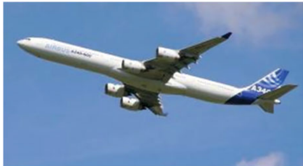
Fig. 13.6 Airbus A340-600 with a maximum take-off weight of 370 t (Photograph [8])
