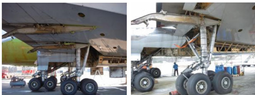
Fig. 14.17 Inner and outer landing gear groups with cylinder and struts
