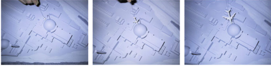
Fig. 13.9 Approach to a nuclear power plant with the three aircraft models Phantom, Airbus A320 and Boeing 747 in a size comparison
