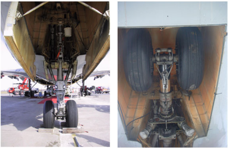
Fig. 14.15 Nose landing gear; on the left in the extended position, on the right in the retracted position; the hydraulic cylinder points forward in the direction of flight
