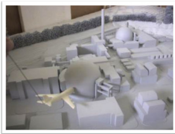
Fig. 13.10 Possible approach zone to the cylindrical part of a convey containment; situation with a true to scale model of a Boeing 747
