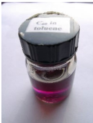
Fig. 3 A solution of C 60 , the first ever soluble form of carbon (picture Jonathan Hare)
