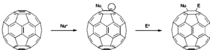
Scheme 1 Generic schematic of nucleophilic attack of C_{60} followed by quenching by electrophile
