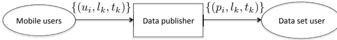
Fig. 1. Pseudonymized location data publishing. The data publisher replaces a user’s identity u_i with a pseudonym p_i before releasing location data to data set users.
