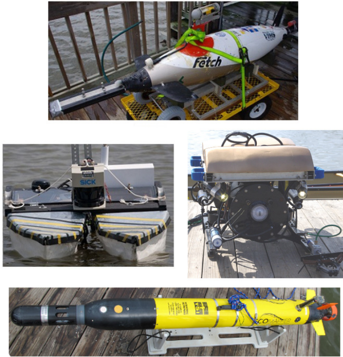
Fig. 1. Marine vehicles used in the survey. From top to bottom: AUV-Fetch1, ASV-Victoria (left), ROV- \beta (right), and the AUV-EcoMapper.
