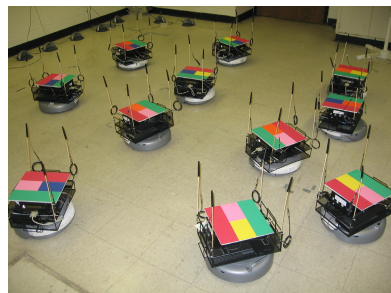
Fig. 15. MiNT Testbed with mobile robotic nodes [6]
