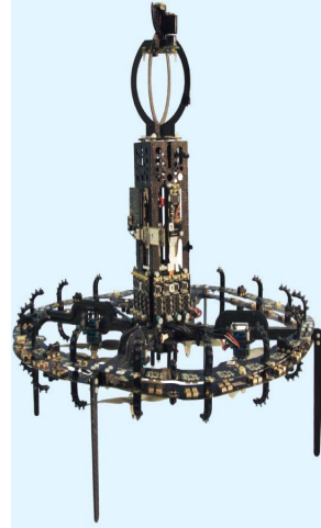
Fig. 12. Autonomous flying robot, eyebot, to explore indoor environments [8]
