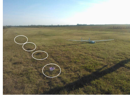
Fig. 12. Preliminary field experiments of WSN data collection using a UAV performed in October 2012
