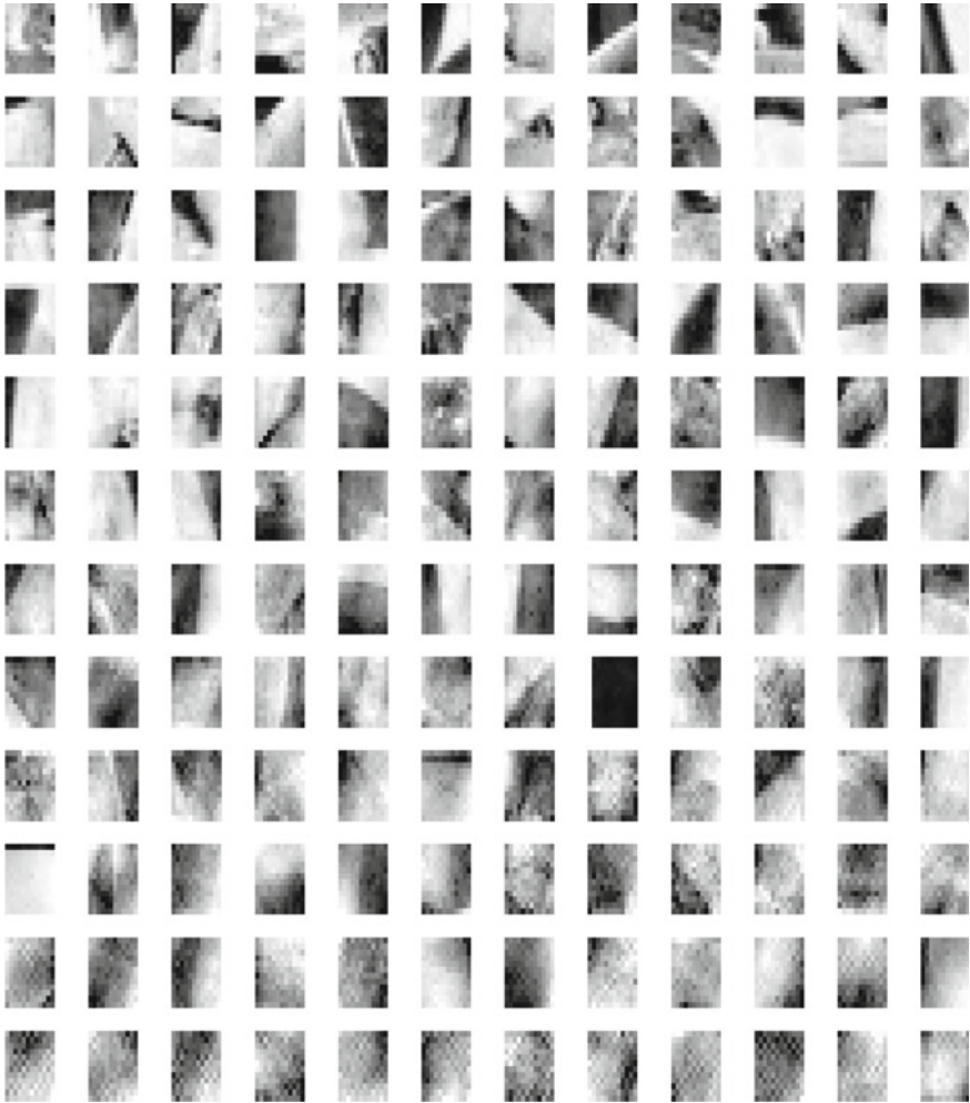
Fig. 16.10 Typical ICA image-basis obtained from 12 \times 12 patches
