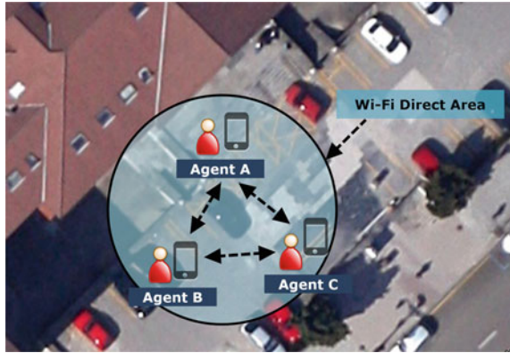
Fig. 1 Conceptual scheme, three intelligent agents geographically close obtains the GPS location and share it with nearby agents using a Wi-Fi Direct connection
