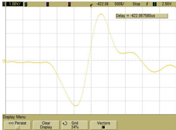
Fig. 7 Actual measurement of the bipolar UWB pulse
