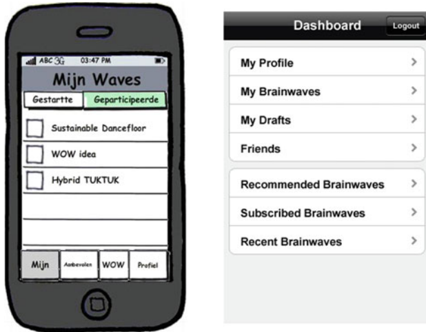
Fig. 10. A paper prototype or a user interface sketch (left) to present test-users or other designers what a design will look like. On the right a clickable prototype to present the interaction design or user-system dialogue of a smartphone application.
