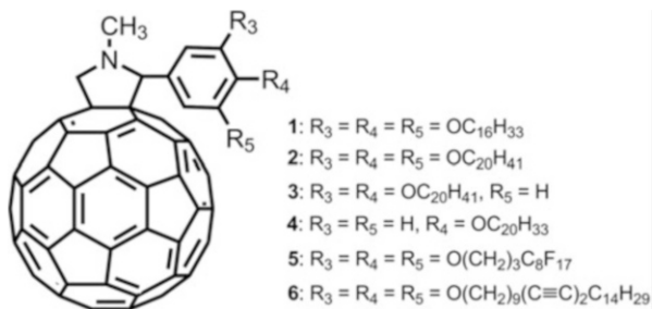
Scheme 2 Chemical structures of alkyl-conjugated C_{60} derivatives 1–6
