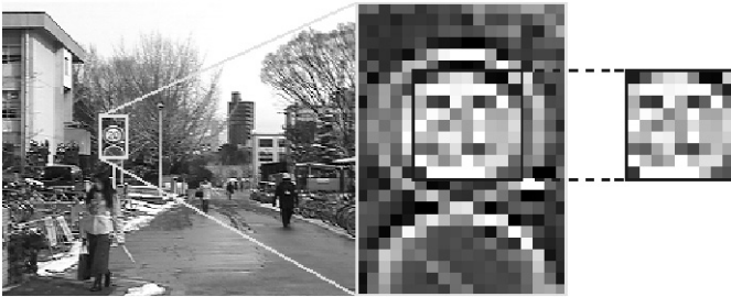
Fig. 2 A traffic sign symbol extracted from an actual image taken by a digital video camera
