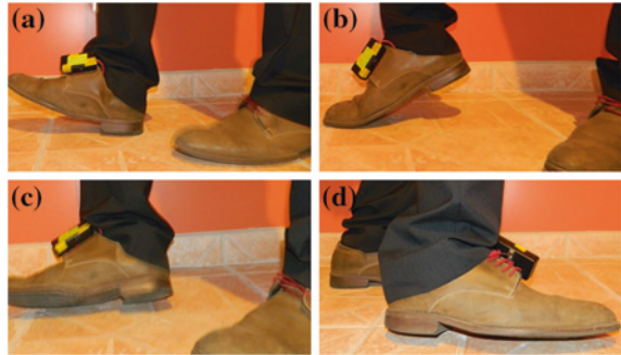
Fig. 20.4 Gestures used for the accelerometer based metaphor. a Forward. b Backward. c Rightward. d Leftward
