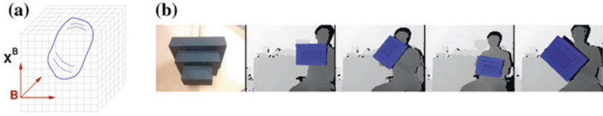
Fig. 16.3 a The voxelized space around an object. In practice the volume is 384 \times 384 \times 384 voxels. b An object being tracked during calibration. The calibration parameters converged after some 300 frames, or 10 s of movement
