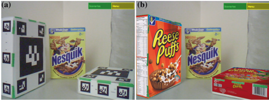
Fig. 22.1 A simple augmented reality example. a Original video feed. b Augmented scene
