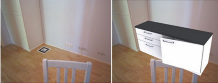
Fig. 22.3 Unrealistic effects are created in cases in which augmented objects occlude real objects. In this picture the drawer should be rendered behind the chair
