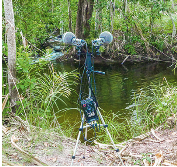
Fig. 26.2 Field recorder and stereo microphones on tripod, recording bird and water sounds
