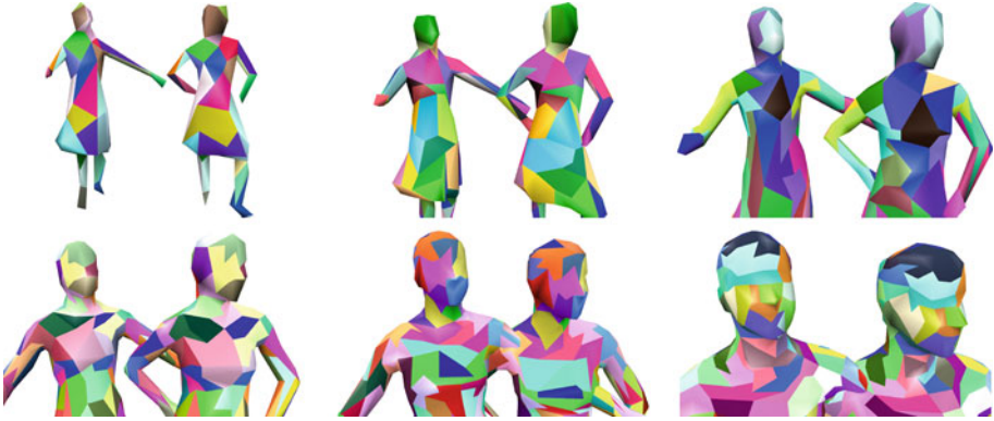
Fig. 5. Multiresolution Framework. The images show matchings between two shapes at different resolutions. As described in Sect. 5 the computational cost is drastically reduced by first solving the matching problem at a lower resolution and then using the obtained solution to restrict the search space at the next higher resolution.
