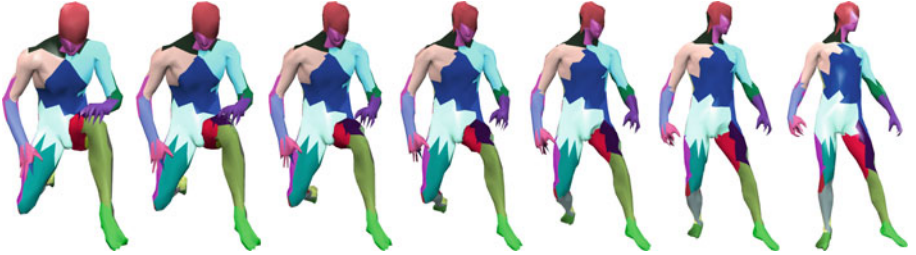
Fig. 7. Linear Interpolation. The images show a matching between the leftmost and rightmost models taken from the SHREC 2011 benchmark [28] by linearly interpolating between the triangle correspondences. This transition illustrates the geometric consistency property of the proposed method: At any time during the interpolation the model is a closed triangle mesh.
