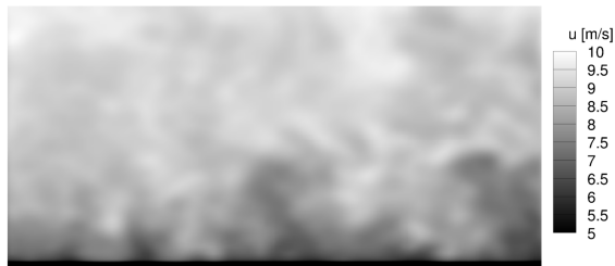
Fig. 1 Extract of LES data provided by DEWI; The data were extracted in a yz -plane at a specific time step; Several time steps are used as inflow data for the simulations; The data provides velocities up to 10 m/s and has yaw included
