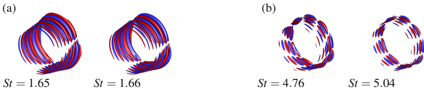
Fig. 7 (a) Energetic low frequency group structures (modes) and (b) energetic high frequency group structures of the linear subdomain
