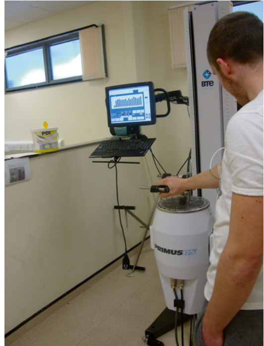
Fig. 44.1 Denervation test is done by assessing wrist function, pain and work output, which is measured before and after a local anaesthetic block. Decrease in pain by 75–90 % and a doubled increase in work output predict a good outcome after denervation
