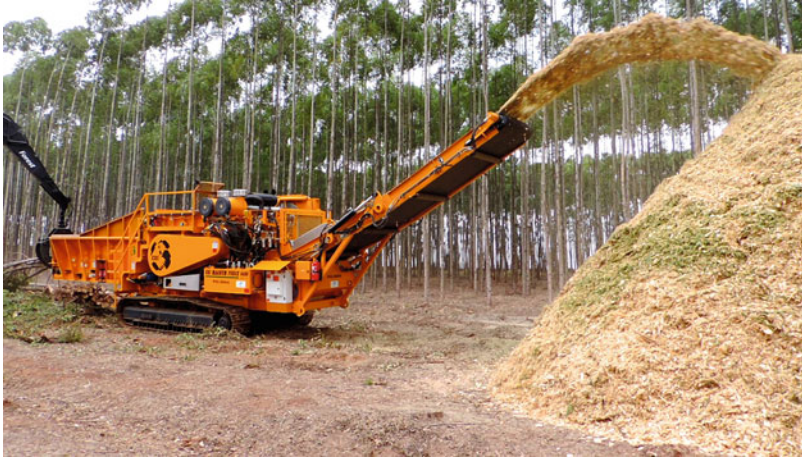
Fig. 41 Self-driving grinder (remote control) for stumps removing in forest plantations. Source: Gustavo Castro
