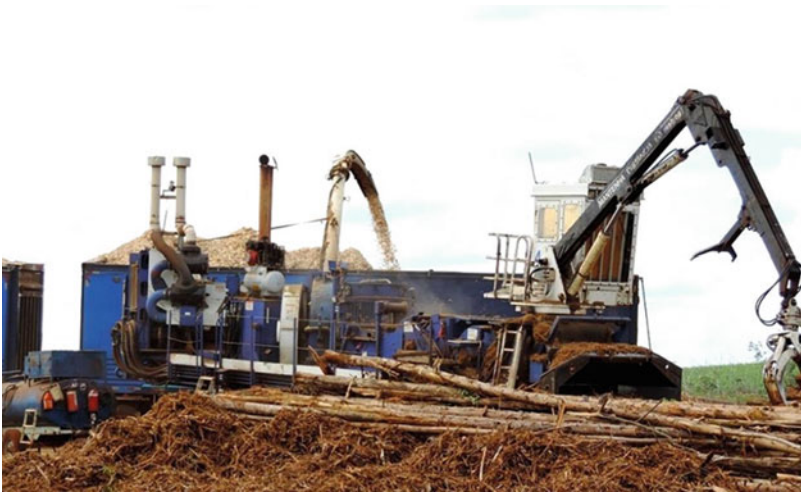
Fig. 40 Mobile drum chipper in a forest plantation. Source: Gustavo Castro
