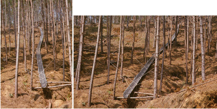
Fig. 20 Wood extraction with chutes. Short log extraction in a pine plantation ( left ) and schematic drawing ( right ). Source: Jorge Malinovski
