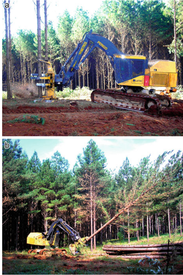
Fig. 14 A feller buncher grabbing a tree ( top ) and felling and bundling it ( bottom ). Source: Gustavo Castro
