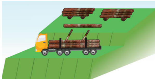
Fig. 46 Ramp on the upper side of a batter that might be constructed in mountainous terrain. Source: The authors
