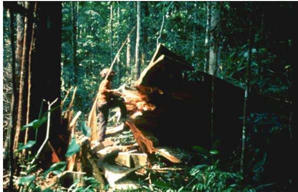
Fig. 4 Motor-manual felling with chainsaw in the Amazon region. Source: Grammel. Source: Grammel
