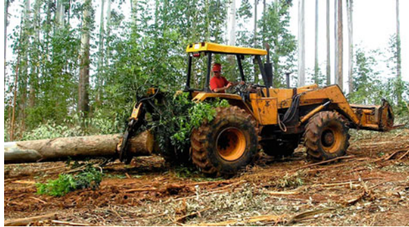
Fig. 27 Mini-Skidder, an adapted agricultural tractor in a forest plantation. Source: Gustavo Castro
