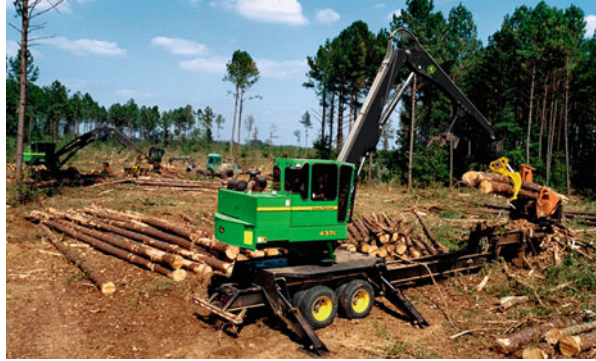
Fig. 47 Multifunctional knuckle boom loader mounted on a trailer. Source: John Deere Forestry
