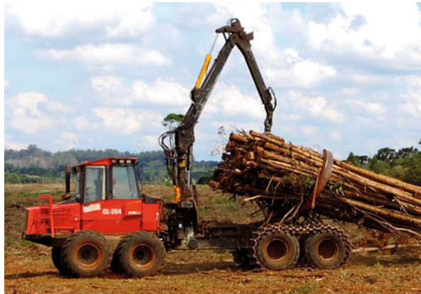
Fig. 32 A clambunk skidder in a forest plantation. Source: Gustavo Castro
