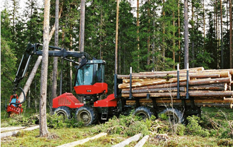
Fig. 34 Wheel-based forest tractor equipped with a crane for felling, delimiting, bucking, and loading as well as with a load carrier for off-road transport (combination of harvester and forwarder, harwarder). Source: Komatsu Forest
