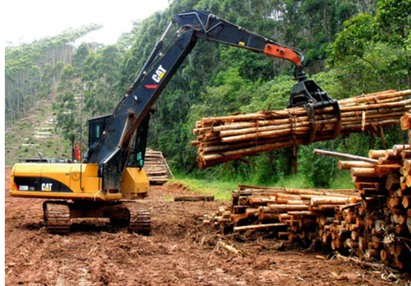
Fig. 48 A log loader mounted on a track-based excavator machine. Source: Gustavo Castro
