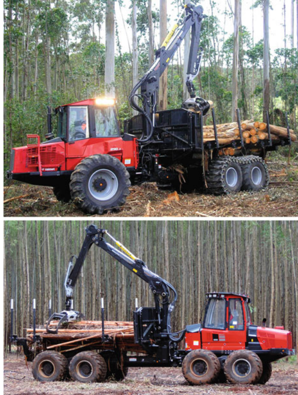
Fig. 33 Forwarder of different sizes with six wheels ( top ) and eight wheels ( bottom ). Source: Gustavo Castro
