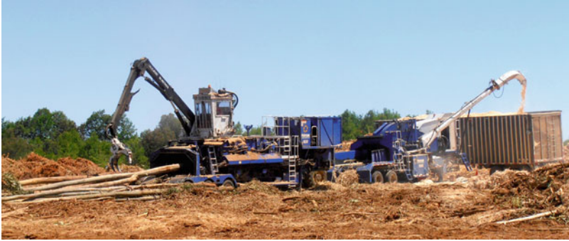
Fig. 39 A combined machine for feeding, delimiting, debarking, and chipping. Source: Gustavo Castro
