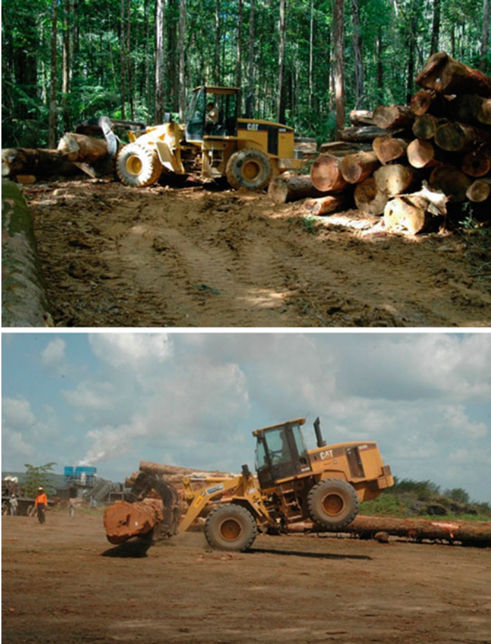
Fig. 49 Wheel front-end loader in the landing zone of a tropical rainforest ( top ) and at the log yard of a sawmill ( bottom ). Source: Leif Nutto
