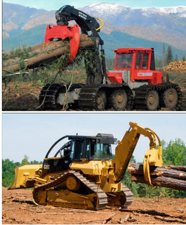
Fig. 30 Eight-wheel skidder with assisting tracks ( top ) and a track skidder ( bottom ). Source: Tanguay / Caterpillar
