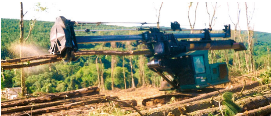
Fig. 15 A stroke delimeter for cutting off branches in a planted forest. Source: Gustavo Castro
