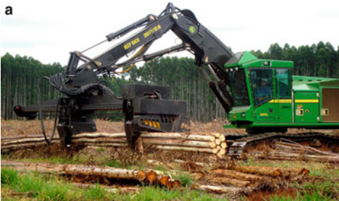
Fig. 11 Big-sized multiprocessing harvester heads ( left ) and a small-sized head for multiprocessing ( right ). Source: John Deere
