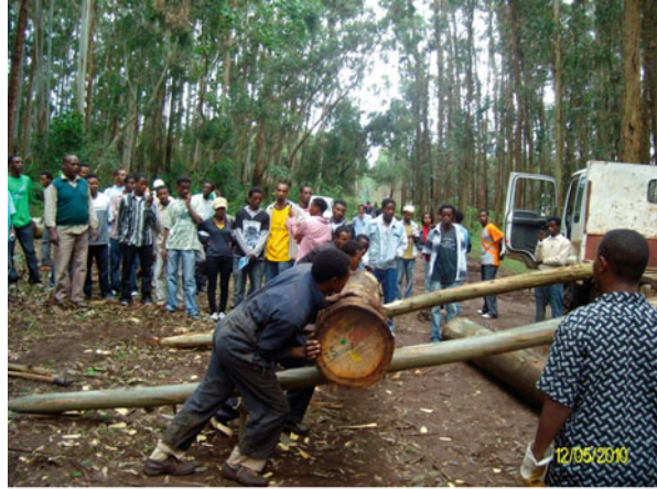
Fig. 43 Extremely dangerous manual loading of eucalypt logs under wet and slippery conditions in Ethiopia. Source: Leif Nutto
