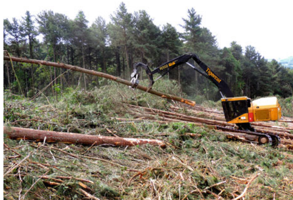
Fig. 35 A shovel logger working in a conifer planted forest. Source: Gustavo Castro
