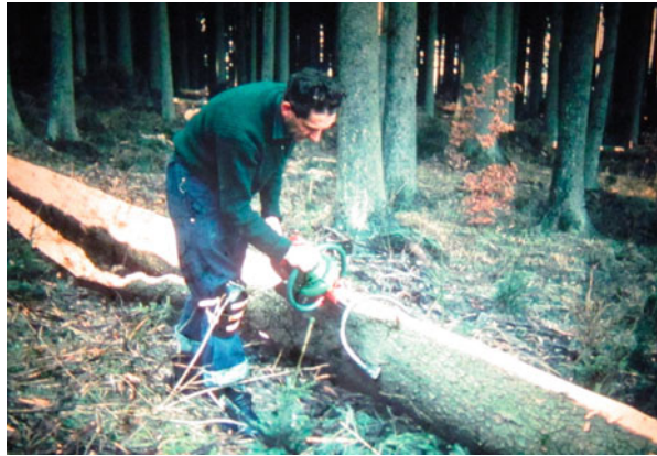
Fig. 6 Motor-manual debarking of logs with a tool mounted on a chainsaw. Source: Jorge Malinovski
