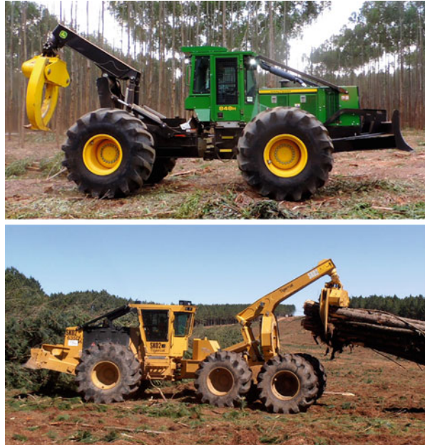
Fig. 29 Grapple skidder with four wheels ( 4 \times 4 , top ) and six wheels ( 6 \times 6 bottom ). Source: Gustavo Castro
