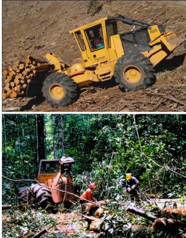
Fig. 31 Skidders equipped with a winch in forest plantation ( top ) and in a native forest ( bottom ). Source: Tigercat / Leif Nutto
