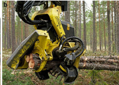
Fig. 11 Big-sized multiprocessing harvester heads ( left ) and a small-sized head for multiprocessing ( right ). Source: John Deere
