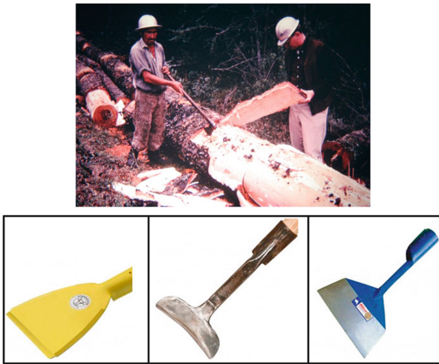
Fig. 2 Manual debarking with ax and different-shaped hand tools for manual debarking. Source: Leif Nutto
