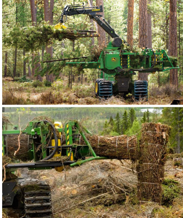
Fig. 42 Slash bundler for compacting crown slash for transport. Source: John Deere Forestry
