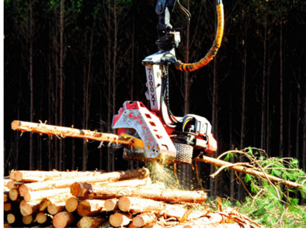
Fig. 16 A processor head processing (debarking, delimiting, and bucking) trees at the road side. Source: Gustavo Castro
