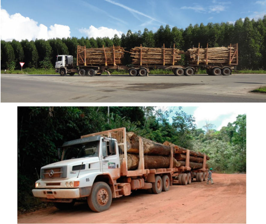
Fig. 3 Pulpwood transport with road train ( left ) and stem transport coming from native forest harvesting in the Amazon ( right ). Source: Gustavo Castro / Leif Nutto
