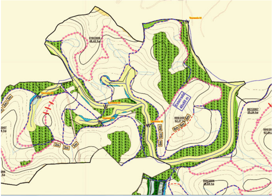
Fig. 11 Thematic map for microscale planning, containing all details like restricted area, water bodies, forest roads, contour lines, landing zones for wood piles, slope of roads, and terrain. Source: Cenibra
