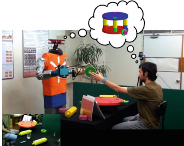
Fig. 13.2 Joint action scenario: the human-robot team has to assemble a ‘toy vehicle’ from components that are initially distributed on a table
