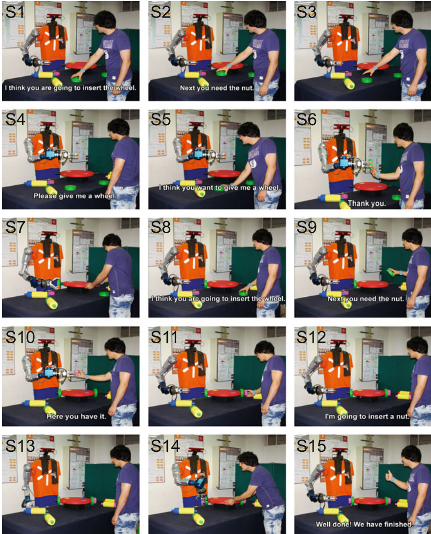
Fig. 13.4 Video snapshots that illustrate the capacity of the robot to infer goals, take initiative and anticipate the user's future needs
