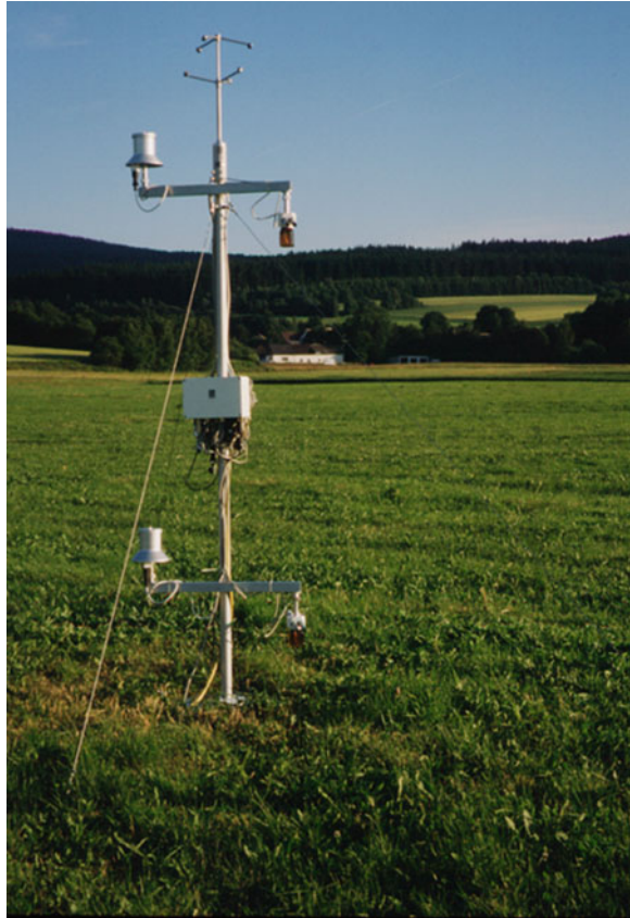
Fig. 7.4 Modified Bowen-ratio system for sensible and latent heat flux according to Liu et al. (2001), Photograph by Foken
