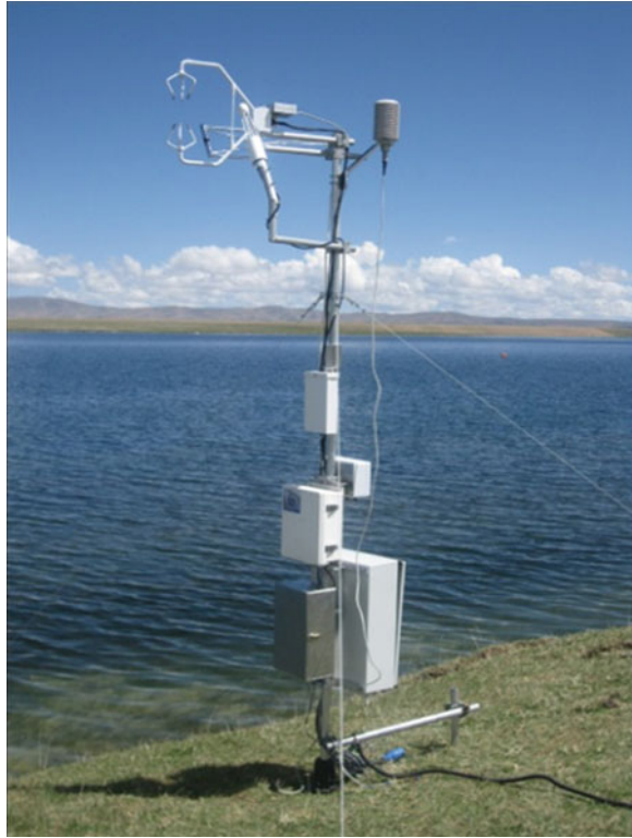
Fig. 7.10 Measuring complex for eddy-covariance measurements consist on a sonic anemometer CSAT3 and an IR gas analyser LiCor 7500 (Photograph by Foken)
