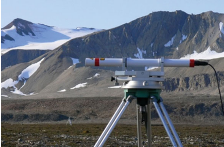
Fig. 7.13 Small aperture scintillometer DBSAS, receiver unit, at Svalbard, Norway. The laser source is about 20 m away in the background ( Photograph by Lüers, Published with kind permission of © Dr. habil. Lüers, 2012. All Rights Reserved)
