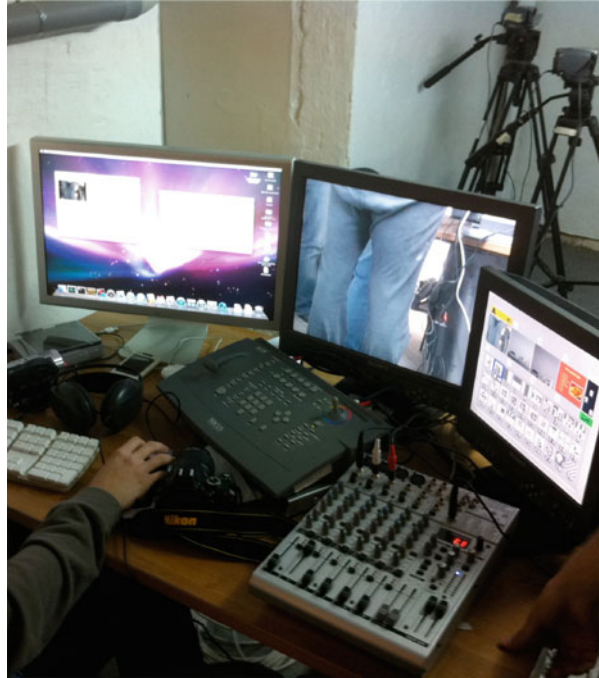
Fig. 2 The iMediaTV control panel featuring the audio mixer, the video mixer, the server and cameras that connects to the video mixer and the direct video server
