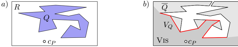
Fig. 2. a) A simple polygon Q and a rectangle R enclosing both c_P and Q . By removing Q from R we obtain a polygon with one hole. b) The simple polygon \bar{Q} obtained by connecting the hole with the boundary of R . In red, the visible chain V_Q of \bar{Q} from c_P .
