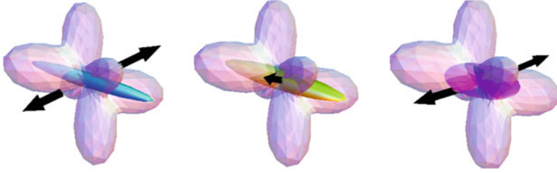
Fig. 2 Illustration of the directional dependency of tensors g_{\alpha\beta}(\mathbf{x}, \mathbf{y}) . The \tilde{P}_4(\mathbf{x}, \mathbf{y}) profile is shown as a surface in all images. The arrows indicate specific directions \mathbf{y} , and the ellipsoids represent the tensors g_{\alpha\beta}(\mathbf{x}, \mathbf{y}) calculated from \tilde{P}_4(\mathbf{x}, \mathbf{y}) by fixing the direction \mathbf{y} for each image
