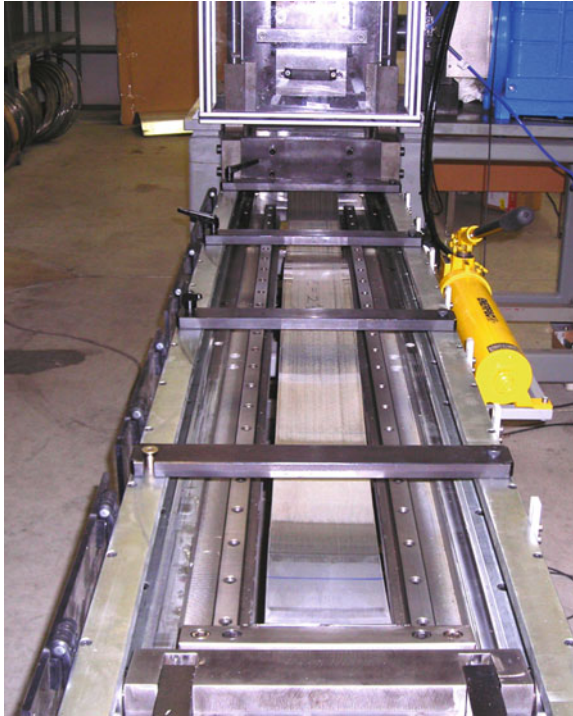
Fig. 4 Equipment developed for implementing a continuous process of plastic deformation by angular channel for manufacturing sheet, based on the patent proposed by Luis et al. (Pat. 2224787, 2002) [1]. The prototype is installed in the facilities of the Department of Mechanical, Energetics and Materials Engineering from the Public University of Navarre
