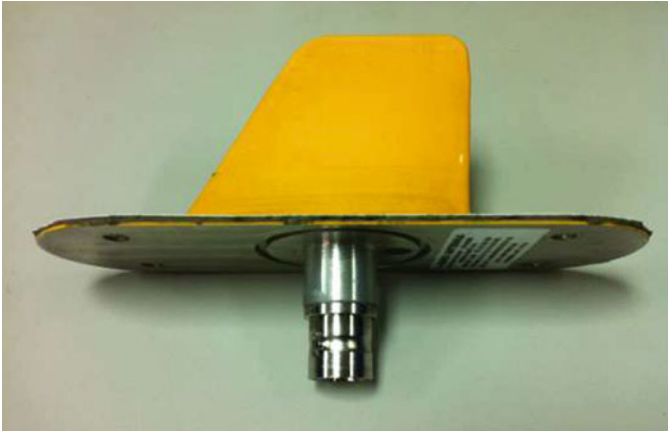
Fig. 43.5 A failed ATC antenna (only used 3 months on brand-new airplane)
