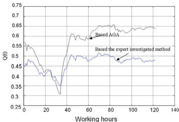
Fig. 12.4 Fixed weights based on genetic algorithm and the integrated parameters change over time
