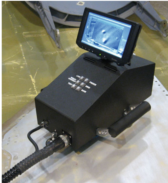
Fig. 5.3 Shearography test on aluminum honeycomb panel
