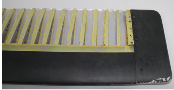
Fig. 37.2 The helicopter rail rotor blade with debonding damages
