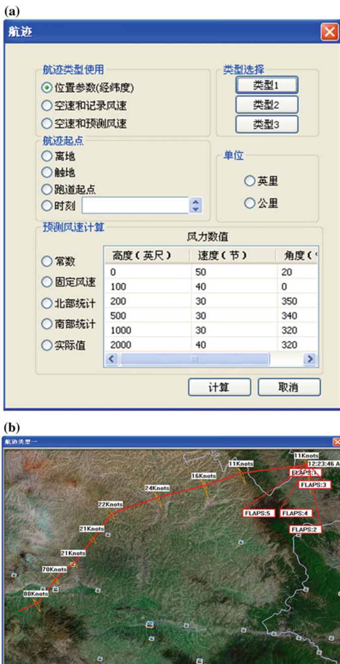
Fig. 39.9 a The parameter selection screen. b Aeronautical charts plotted interface
