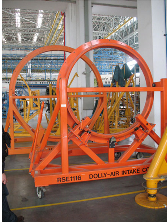
Fig. 36.10 RSE1116 bracket (front view)
