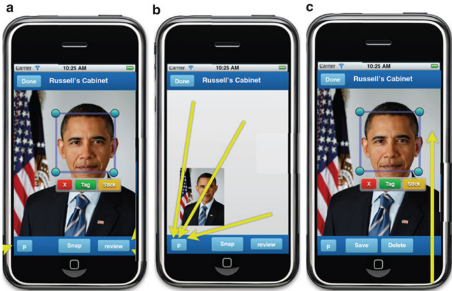
Fig. 4 HyperSite image live tagging mode: (a) Image hyper region, (b) Camera roll, (c) Shoot and review tagging screen, (d) Defined tags option, and (e) Add tag screen
