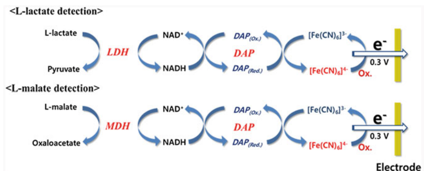
Fig. 9 Schematic illustration of a cascaded bienzyme reaction employed in an electrochemical L-lactate/L-malate biosensor suggested by Katrlík et al. [73]. DAP , Diaphorase; LDH , Lactate dehydrogenase; MDH , Malate dehydrogenase; NAD , Nicotinamide adenine dinucleotide (oxidized); NADH , Nicotinamide adenine dinucleotide (reduced)
