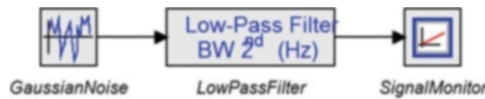
Fig. C.15 A low-pass filter being used to attenuate the noise from a Gaussian noise source.
