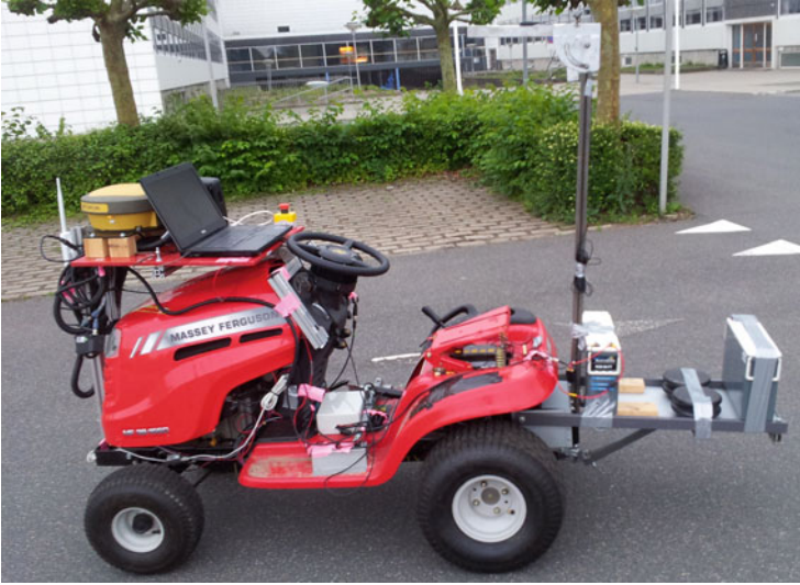
Fig. 10.8 ASuBot: a Massey Ferguson 38-15 garden tractor retrofitted with a Topcon AES-25 steering system
