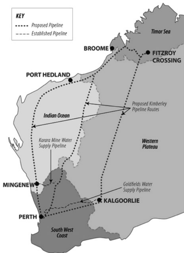
Fig. 14.1 Western Australia’s water pipelines (Adapted from Ghassemi and White 2007: 66, 170, 156). The three water pipeline routes from the Kimberley were initially proposed in 1988 to bring water from the Timor Sea basin to the South West Coast basin. The Goldfields Water Supply pipeline was established in 1903 transferring water from the South West Coast basin to the arid Western Plateau. The Karara water pipeline was completed in 2011 and transfers water from the Indian Ocean basin to the northern section of the South West Coast basin
