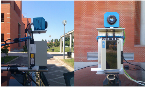
Fig. 1. Laser and infrared camera prototype on-board of the vehicle
