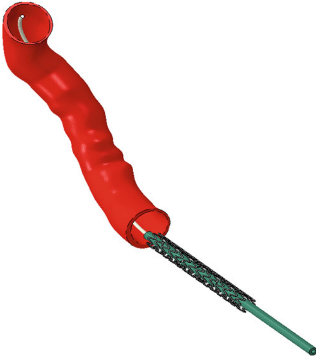
Fig. 5 Patient specific right coronary artery segment. A Boston Scientific Element stent model is also shown before crimping on a catheter, guide-wire system
