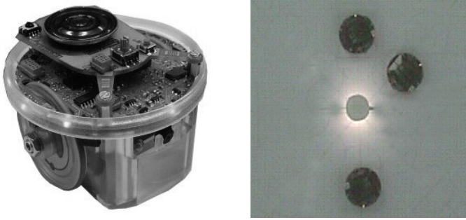
Fig. 14.1 Left: The e-puck robot developed at the EPFL in Lausanne, Switzerland (Mondada and Bonani 2007). Right: A close up view of the environment with the light bulb in the centre and three robots.
