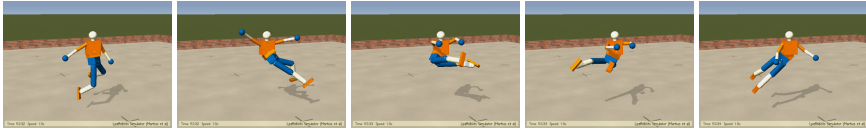
Fig. 7.8 One period of an emerging periodic motion pattern with the trunk fixed and an additional back joint giving the robot more freedom of motion. Coherence is now caused not only by the original symmetries but also by the physical cross-talk becoming “louder” with increasing activity of the robot.
