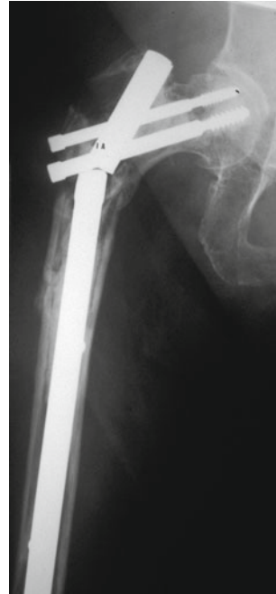
Fig. 25.6 Example of fatigue failure of osteosynthesis. The patient had myeloma affecting the right proximal femur. Intramedullary nail with cement augmentation was used. The patient outlived the implant
