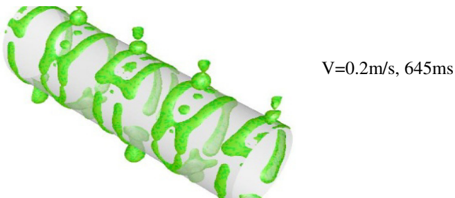
Fig. 2(a). The distribution of liquid film with different flow velocities at entrances of circular tube EP01
