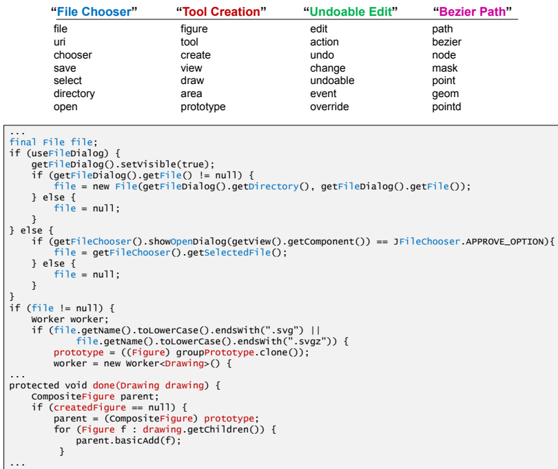
Fig. 5.3: Four example topics (their labels and top words) from JHotDraw 7.5.1. We also show a snippet of the file SVGCreateFromFileTool.java, with terms colored corresponding to the topic from which they came. In this example, no terms come from the “Undoable Edit” or “Bezier Path” topics.
