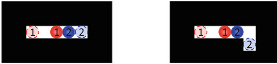
Fig. 2. In this image, black cells are fixed, white cells are free, solid discs are individual particles, and goal positions are dashed circles. For the simple world at left, it is impossible to maneuver both particles to end at their goals. The world at right has a finite solution: \langle r, d, l \rangle .
