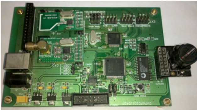
Fig. 9. Wireless video development board
