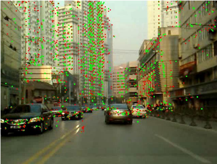
Fig. 4. An image with detected corners (red dots) and suppressed corners (green dots)
