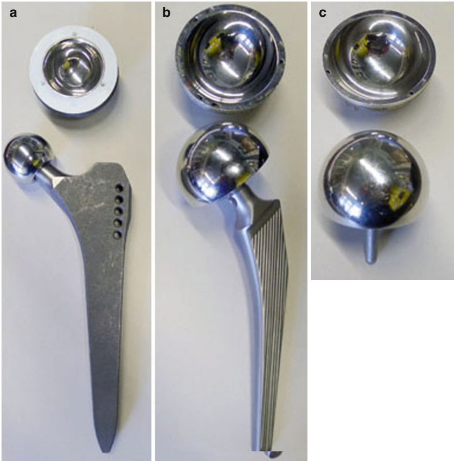
Fig. 1.4 The three different types of MoM THA: (a) Modular small-diameter head ( \leq 32 mm). (b) Modular large-diameter head ( \geq 36 mm). (c) Hip resurfacing arthroplasty (Note: the definition of 36 mm as large is somewhat arbitrary; some sources categorize it as the largest small head)
