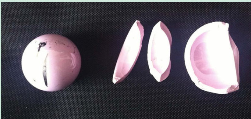
Fig. 10.10 Fractured delta ceramic liner
