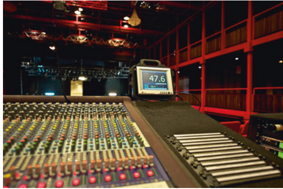
Fig. 1.17 Sound level readout on a laptop computer at the mixing console of Ancienne Belgique, Bruxelles
