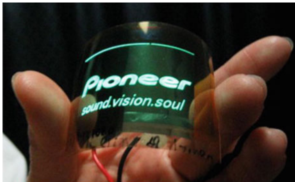
Fig. 15.1 Luminescence of an organic light-emitting diode deposited onto a flexible, low coefficient of thermal expansion (CTE) and optically (Reprinted from Okahisa et al. [17], with permission from Elsevier)
