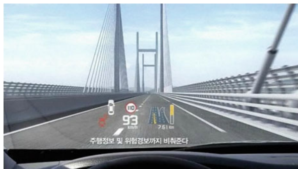
Fig. 21.41 HUD navigation installed in K9 (Kia Motor) for the first time in Korea [56]
