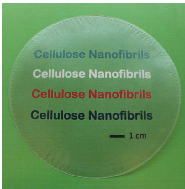
Fig. 15.4 Nanofibrillated cellulose film
