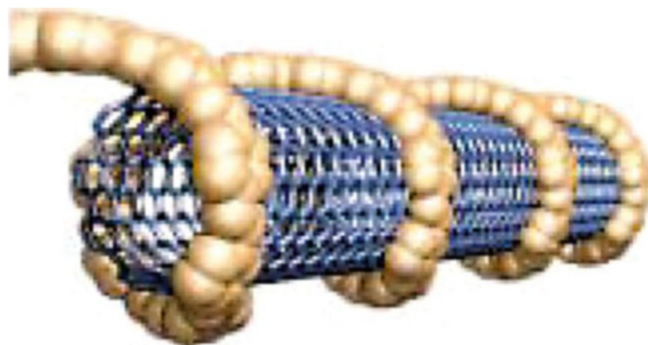
Fig. 23.6 Schematic drawing of the non-covalent wrapping of the polymer chain to SWNT [34]
