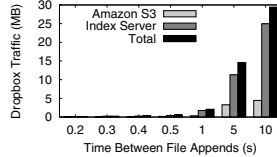
Fig. 7. Dropbox traffic as the time between 1 byte appends is varied (7200 RPM HDD)
