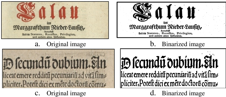
Fig. 2. Binarized output images (b and d) of the original images (a and c) which are classified as SDI
