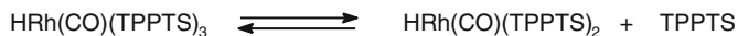
Fig. 12 Coordination–decoordination equilibrium of TPPTS between the non-active [\text{Rh}(\text{CO})(\text{TPPTS})_3] and active [\text{Rh}(\text{CO})(\text{TPPTS})_2] species
