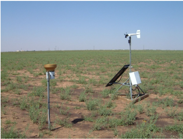
Fig. 2. The automated meteorological tower placed on an experimental site located in a partially vegetated grass field
