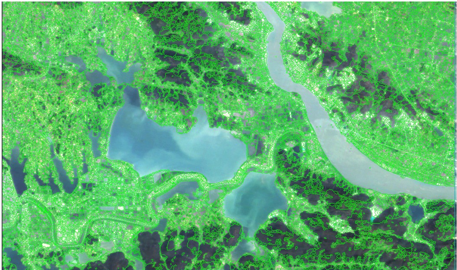
Fig. 4. The Pixels are classified based on the distance between each wave bandy
