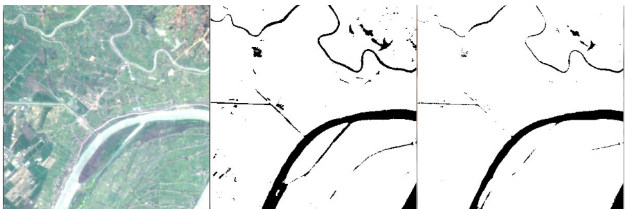
(a) Remote sensing image (b) Water extraction using NDVI (c) Water extraction using NDWI
